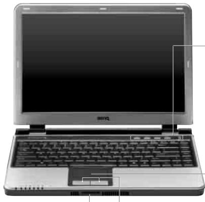
Left and Right Selection Buttons Equivalent to the left and right buttons on a mouse.
